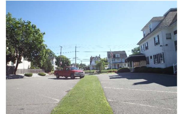
Water currently drains from the parking lot towards the building. The grass buffer in the parking lot can be converted to a rain garden to capture and treat runoff. The sidewalk can be replaced with porous pavement to infiltrate runoff as well. A preliminary soil assessment suggests that soils have suitable drainage characteristics for green infrastructure.
