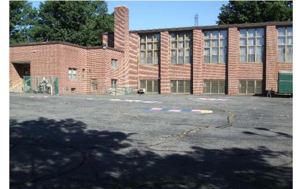
Water on the site currently pools in the parking lot behind the building complex. The lot behind the school can be partially de-paved into a lawn area to address the pooling. Pedestrian walkways can be replaced with porous pavement to capture runoff. A rain garden can also be planted at the back of the site to capture roof runoff and serve as an educational opportunity for students. A preliminary soil assessment suggests that soils have suitable drainage characteristics for green infrastructure.
