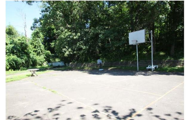
Several disconnected downspouts direct water onto existing porous pavement. A lot of runoff also flows onto the basketball court at the corner of the site, which could be replaced with porous pavement. A preliminary soil assessment suggests that more soil testing would be required before determining soil suitability for green infrastructure.
